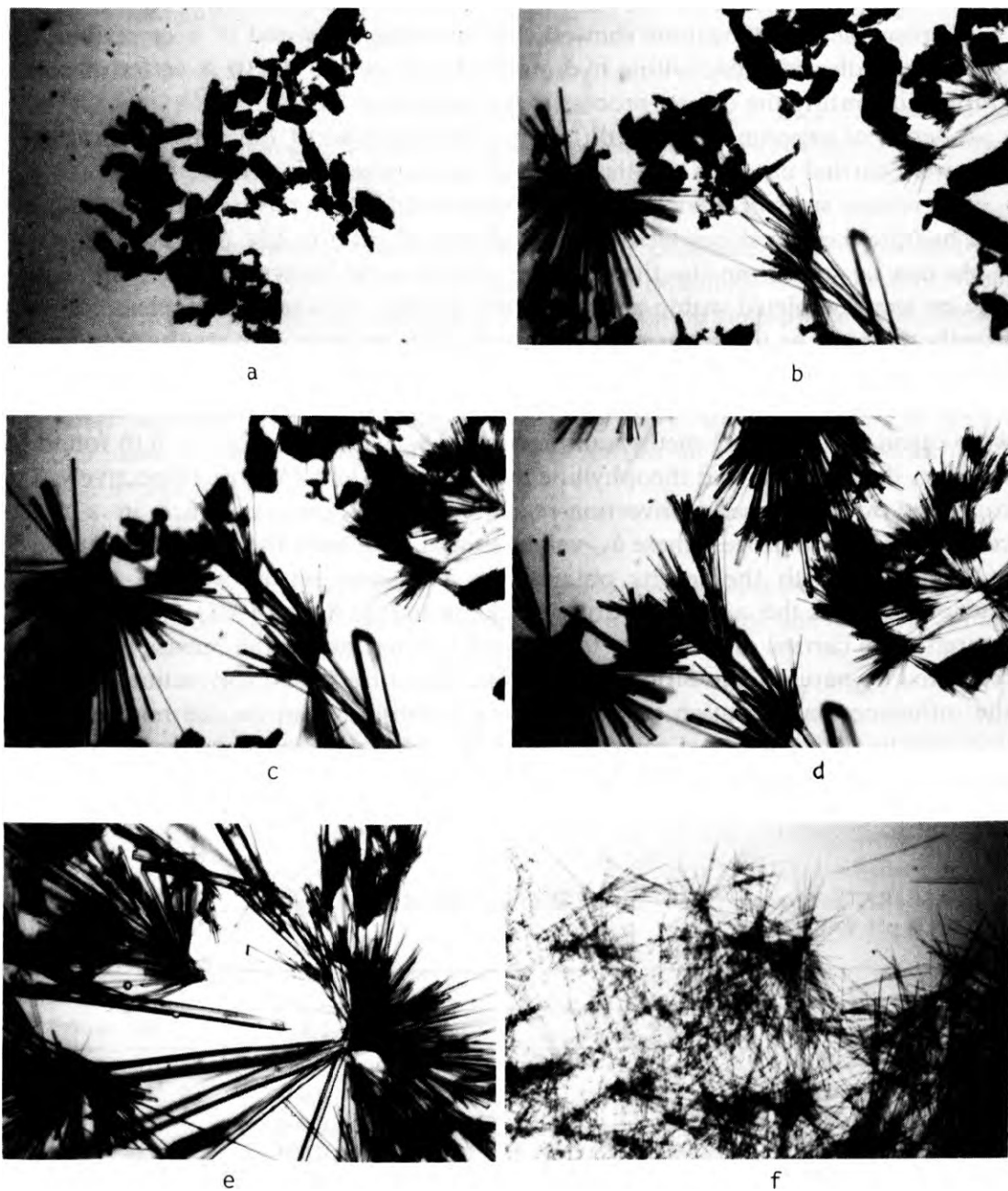
Fig. 4. The crystallization process of theophylline hydrate. a: initial situation: theophylline anhydrate particles in the interface paraffin/buffer pH = 5.0 b-e: the growing process of needles of theophylline hydrate. f: final situation - cake.
